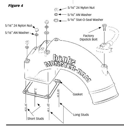
**14.** Slide the second provided intake gasket over the four studs and set the Monster-Ram in place on the studs. Twist a Stat-o-seal washer over the two driverside studs, then over each stud install a flat 5/16" AN washer. Install a 5/16" - 24 nylock nut on each stud and tighten all four evenly between 11-12.5 ft-lb (140 to 150 Inch Pounds) See **Figure 4.**
